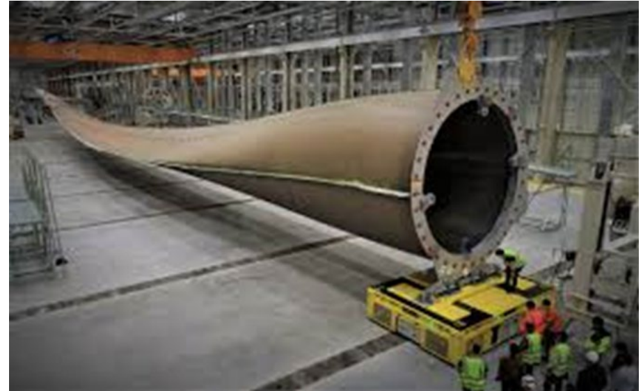
107-meter Blade for GE 12-MW Wind Turbine
