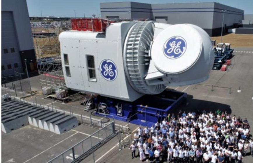
GE 12-MW Wind Turbine Nacelle
